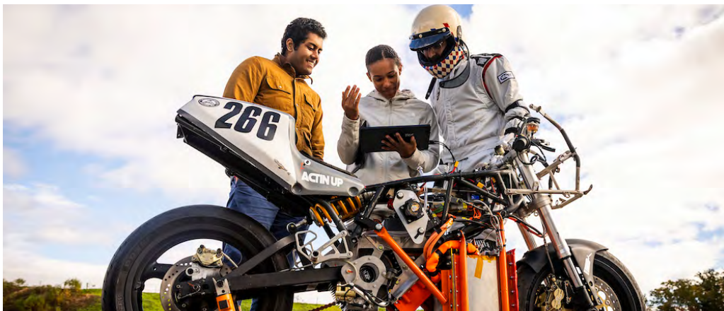
Using an on-board logging computer, Electric Vehicle Team members (left to right) Anand John, Rachel Mohammed, and Aditya Mehrotra check data on the bike's performance, battery levels, and hydrogen tank levels to calculate the range of the vehicle. Photo: Adam Glanzman
