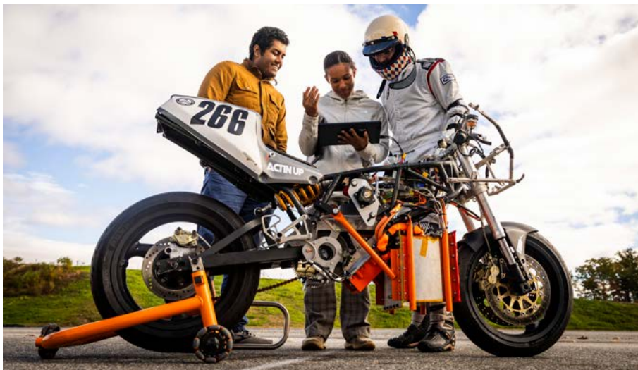
Using an on-board logging computer, Electric Vehicle Team members (left to right) Anand John, Rachel Mohammed, and Aditya Mehrotra check data on the bike’s performance, battery levels, and hydrogen tank levels to calculate the range of the vehicle. Photo: Adam Glanzman
