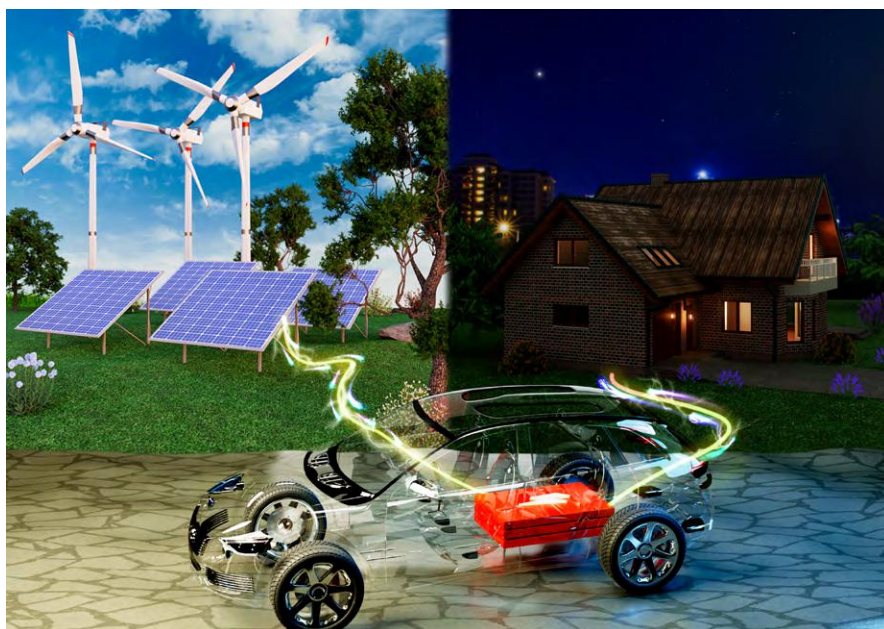
In the future, electric vehicles could boost renewable energy growth by serving as “energy storage on wheels”—charging their batteries from the power grid as they do now, as well as reversing the flow to send power back and provide support services to the grid. Image: Ehsan Faridi and Ehsan Keshavarzi, Inmywork Studio
