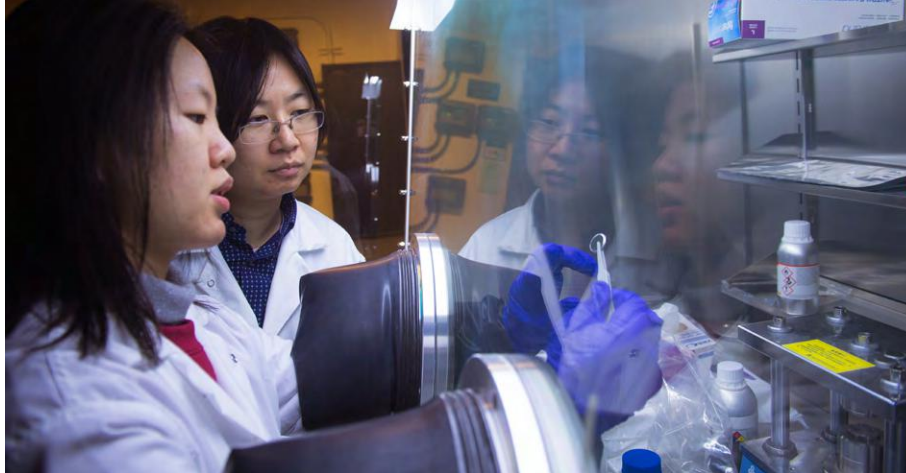
Using a sample of their powders, graduate student Chuwei Zhang (left) assembles a coin-cell battery for performance testing, while Assistant Professor Sili Deng looks on. Working inside a “glove box” is critical because the electrolyte is flammable and the electrodes can degrade in air. Photo: Gretchen Ertl
