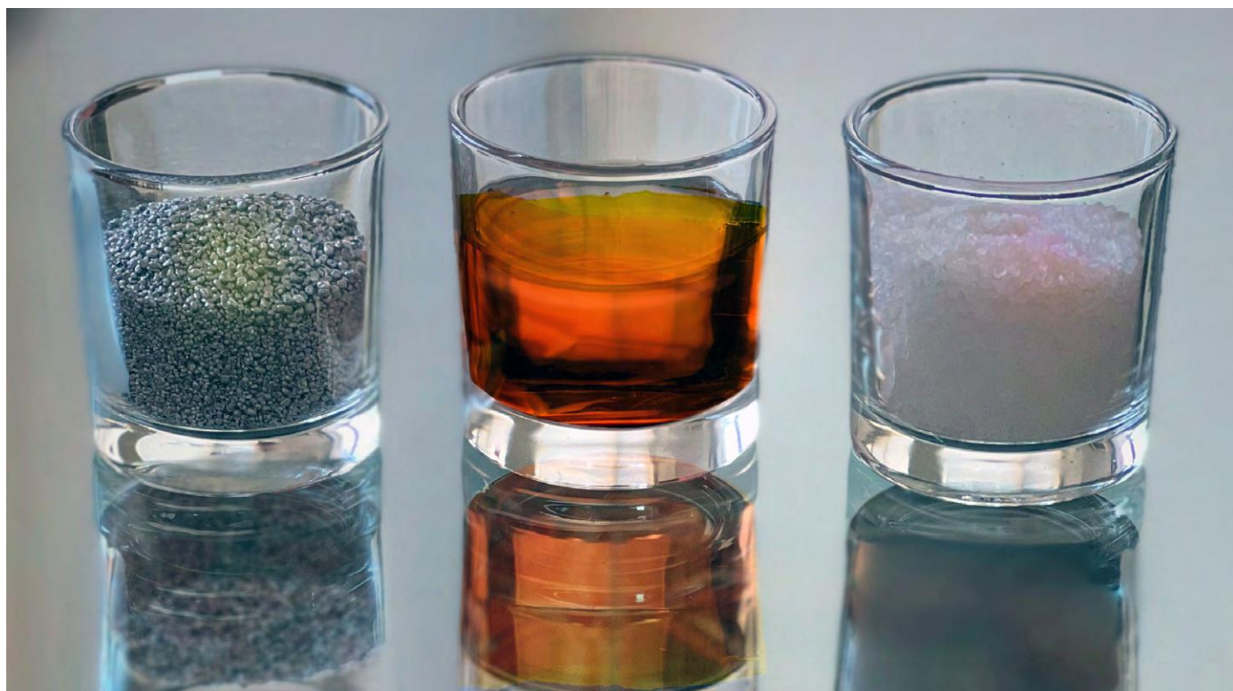
The three primary constituents of the battery are aluminum (left), sulfur (center), and rock salt crystals (right). All are domestically available Earth-abundant materials not requiring a global supply chain. Photo: Rebecca Miller
