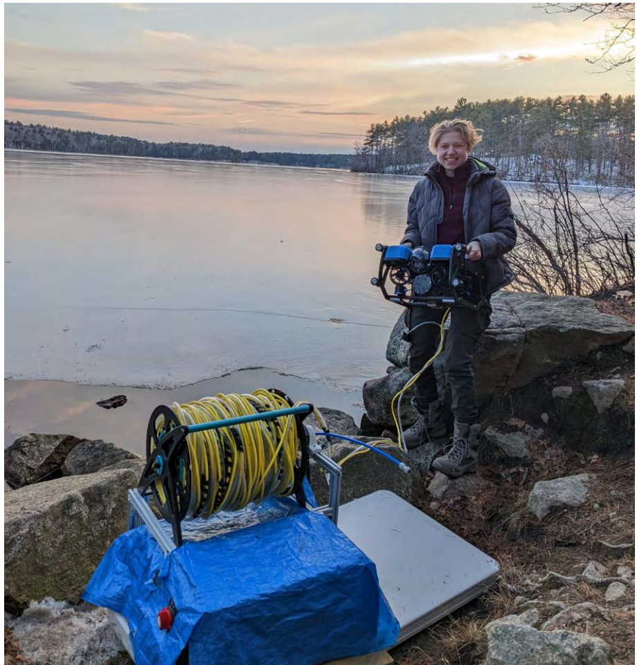
To determine the greenhouse gas emissions from thawing permafrost, MIT senior Sylas Horowitz has been developing a high-performance, remotely operated vehicle (ROV) that can collect water samples from beneath a sheet of Arctic ice. Here, Horowitz field tests the Arctic ROV at Lake Whitehall, Massachusetts. Photo: Victoria Preston
