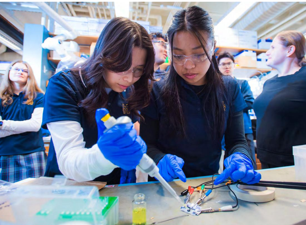
Brianna Tong (left) and Angelina Ang add an electroactive solution to their electrode so that they can measure its conductivity. Next, they will use sophisticated testing equipment in Ariel Furst's lab to see if the electrode successfully conducts electricity. Photo: Gretchen Ertl
