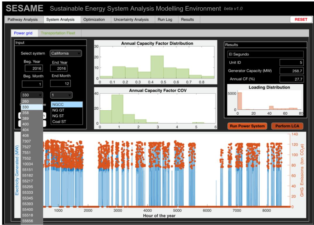
**Figure 7** LCA Results at hourly resolution from El Segundo combined cycle power plant unit 5 is estimated using SESAME’s power system database. The analysis is performed via the Power Grid Systems Analysis tab of the user interface.
