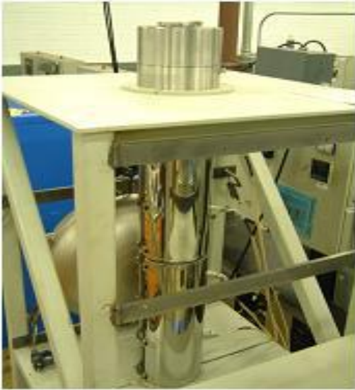
Single Heater Rod WALT Loop Test Facility – at reactor conditions
