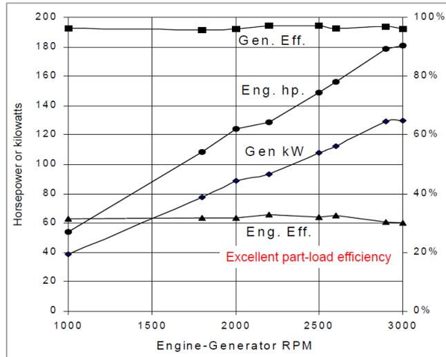
Figure 2: Performance curve for a 100kW Tecogen InVerde Ultra INV-100 model. Source: Tecogen.
