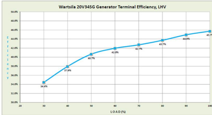
Figure 1: Part-load generator terminal efficiency for a 9.3MW Wartsila 20V34SG model. Source: EPA (2015).
