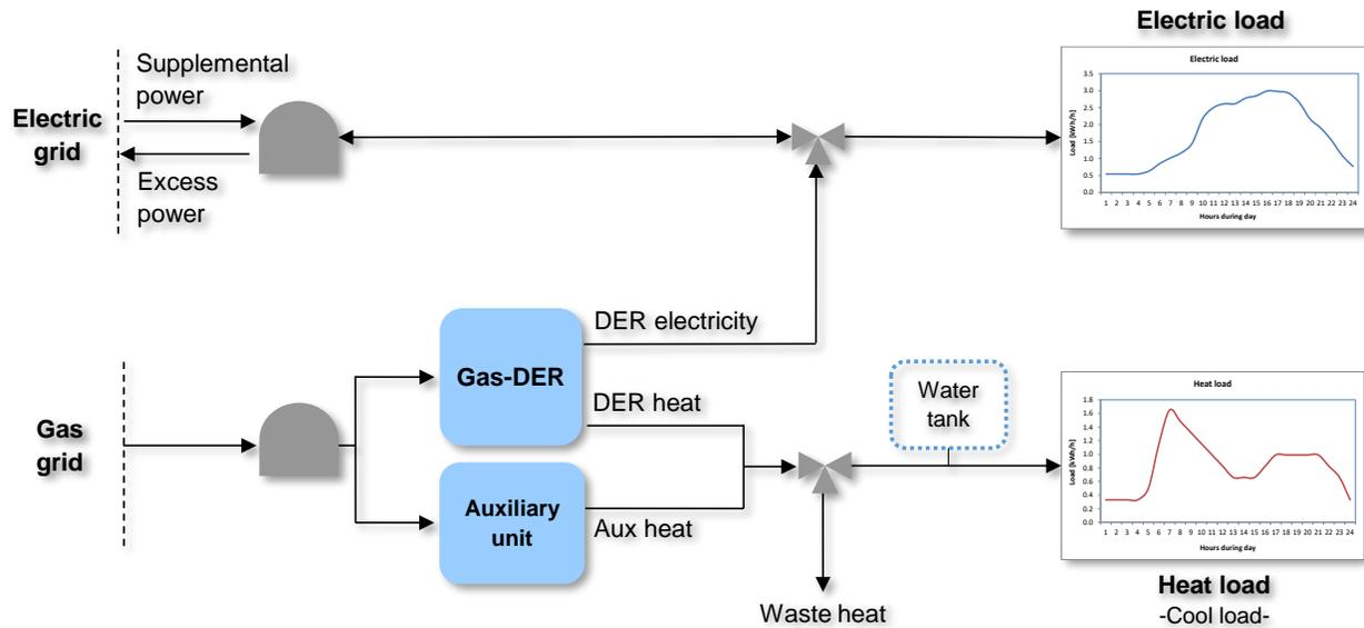
Figure 9: Heating and electric systems using a CHP unit.
