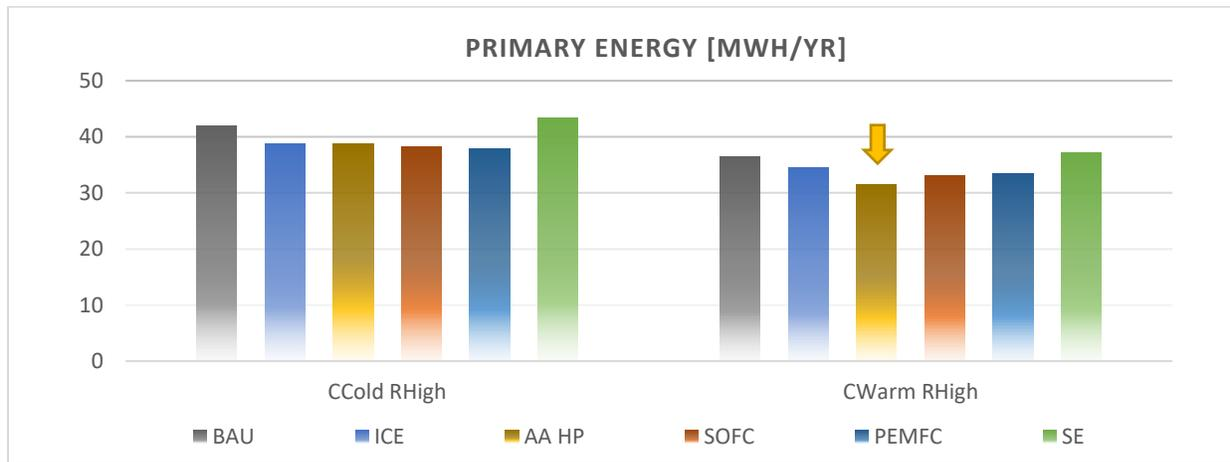
Figure 4: Impact of climate on primary energy of gas- and electricity-based technologies under high electricity-to-gas price ratio.
