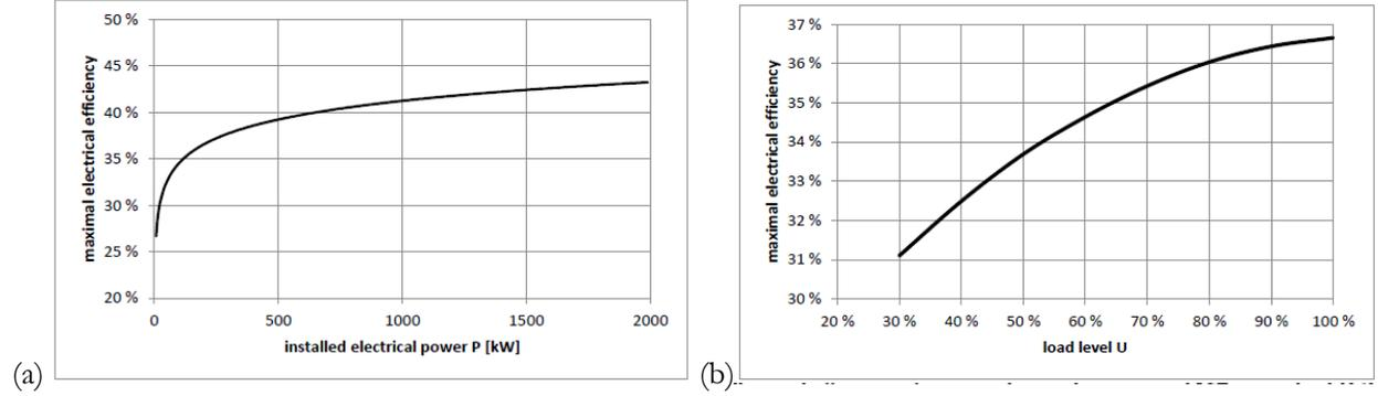
Figure 3: Electrical efficiency as a function of unit size (a) and operating load level (b) for a natural gas-fired ICE. Source: Milan et al. (2015)
