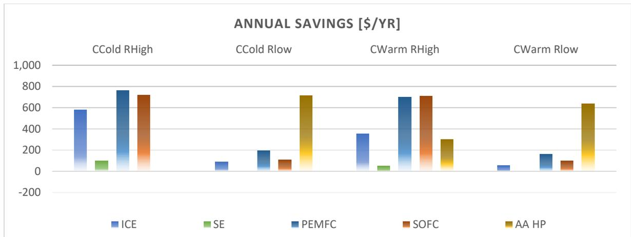
Figure 6: Impact of energy prices and climatic conditions on annual savings of gas- and electricity-based technologies.
