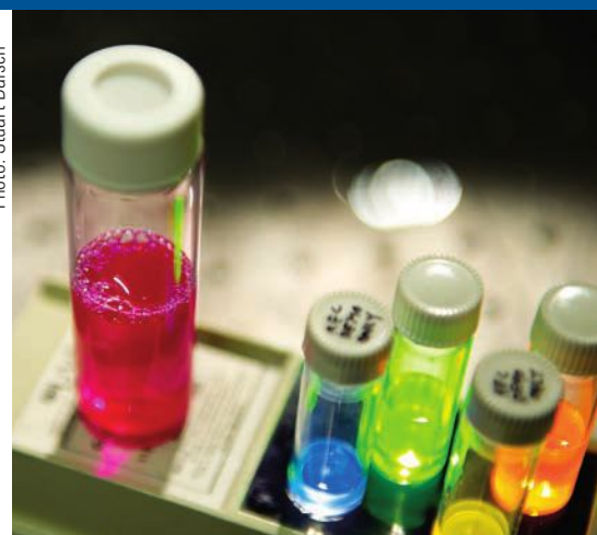
Samples of light-harvesting nanotubes (in the larger vial) and quantum dots that the researchers are synthesizing and studying as they search for novel approaches to collecting, transporting, and using solar energy.
