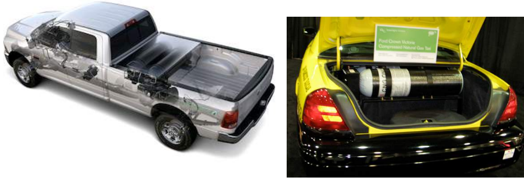
Figure 10. Recently introduced 2012 Dodge Ram 2500 Pickup Truck and Ford Crown Vic taxi cab application. Both pictures show how CNG storage tanks were integrated in vehicle.
