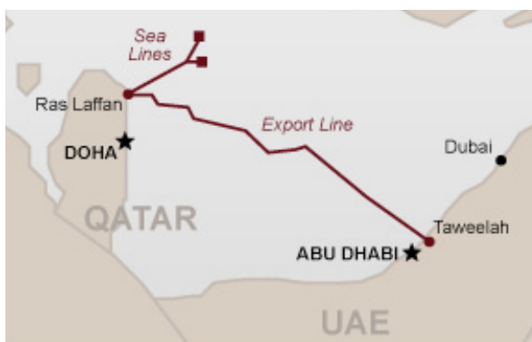
Figure 30: The sea lines transport produced gas from the North Field to the Ras Laffan industrial complex. The export pipeline runs from Qatar to Taweelah in Abu Dhabi, UAE (Source- Dolphin Energy).
