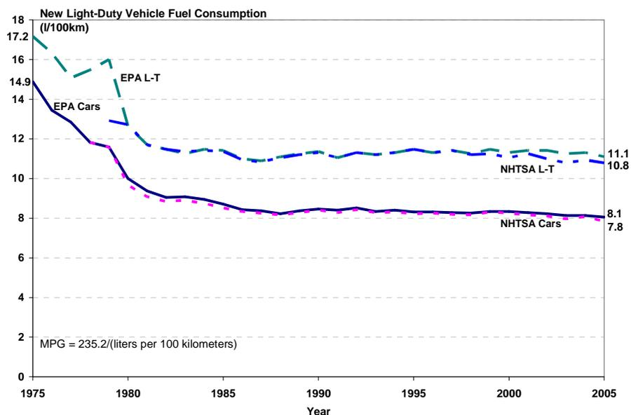
**Figure 27** New light-duty vehicle fuel consumption (1975–2005)
