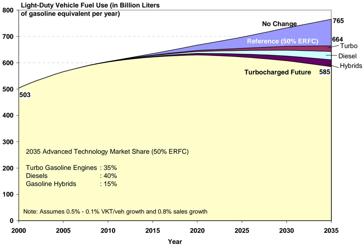
**Figure 56** LDV fuel use under the *Turbocharged ICE Future Scenario*
