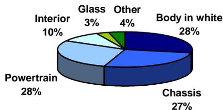
**Figure 14** Vehicle mass distribution by subsystem [Stodolsky et al. 1995]
