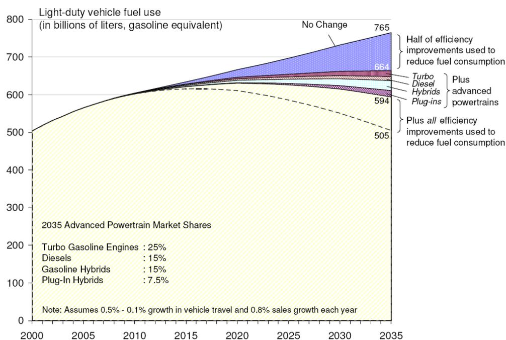
**Figure ES-2:** Representative scenario of light-duty vehicle fuel use with: (i) half of efficiency improvements used to reduce fuel consumption, then (ii) a two-thirds market share of advanced powertrains in 2035, and then (iii) *all* efficiency improvements used to reduce fuel consumption.
