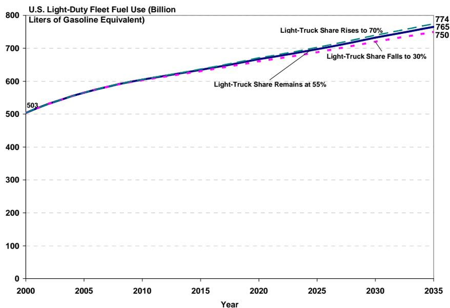
**Figure 32** Effect of new light truck sales fraction on fleet fuel use from 2005 to 2035
