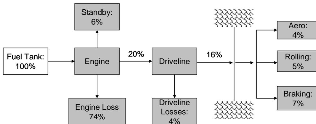
**Figure 9** Representative vehicle energy flows in an urban driving cycle
