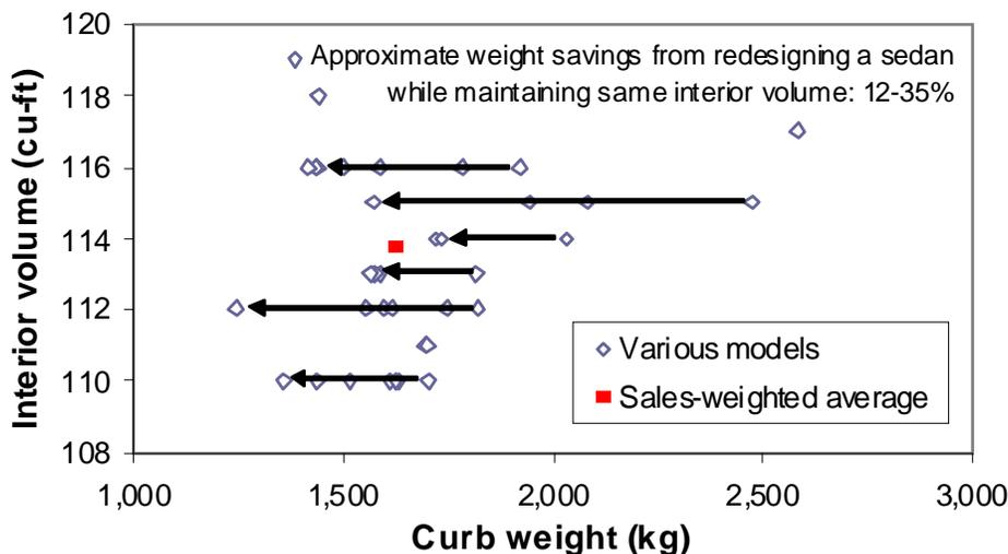
**Figure 16** Potential weight savings from redesigning model year 2007/2008 midsize sedans while maintaining same interior volume
