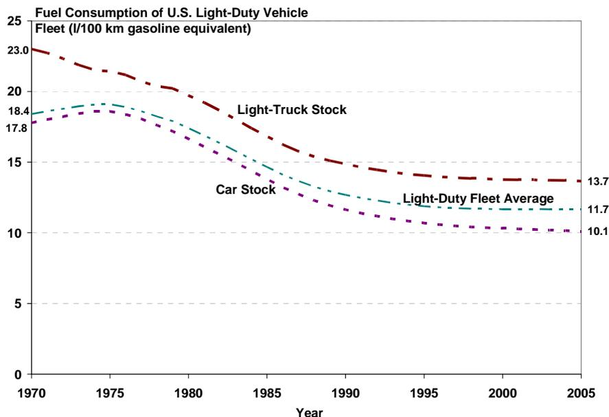
**Figure 2** U.S. Light-duty vehicle fleet fuel consumption (1970–2005)
