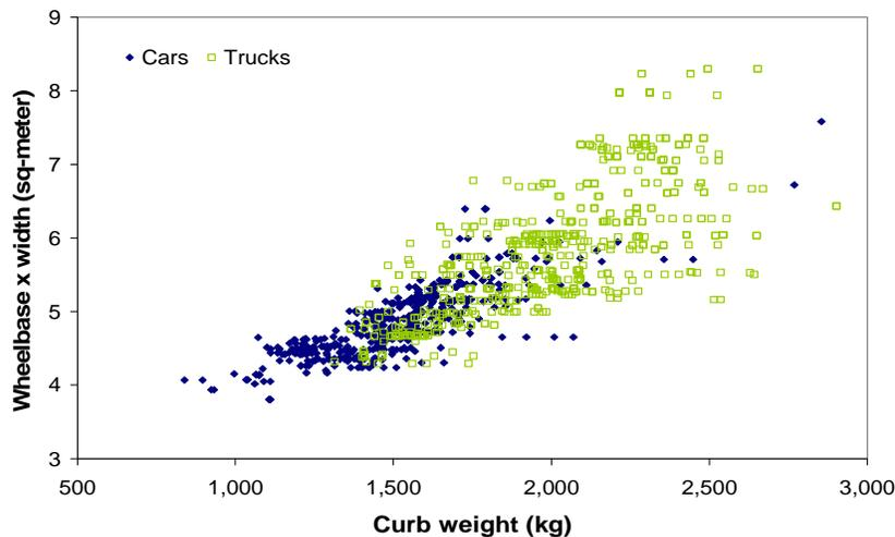
**Figure 17** Size (footprint) vs. weight of U.S. vehicles offered in model year 2005
