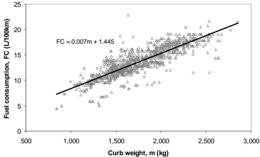
**Figure 12** Curb weight and fuel consumption of U.S. model year 2005 vehicles
