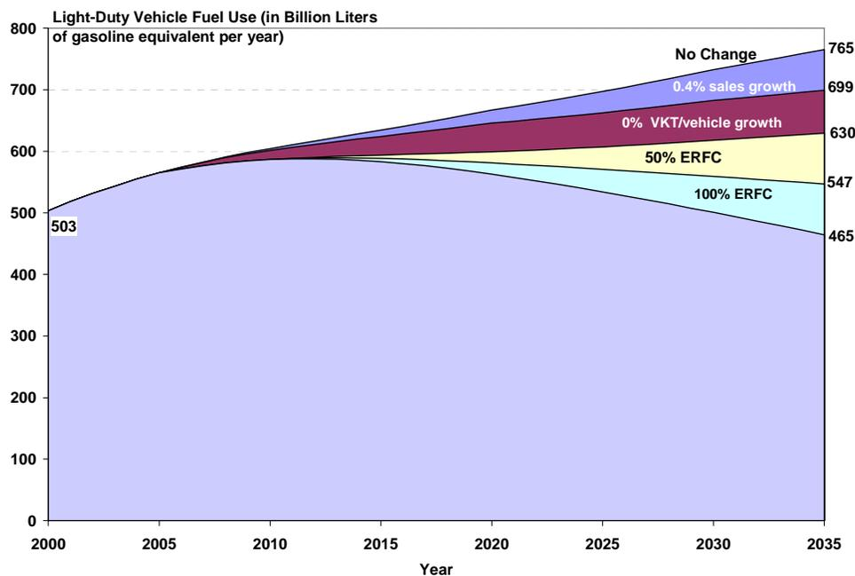
**Figure 67** Effect of reducing rates of growth on LDV fleet fuel use
