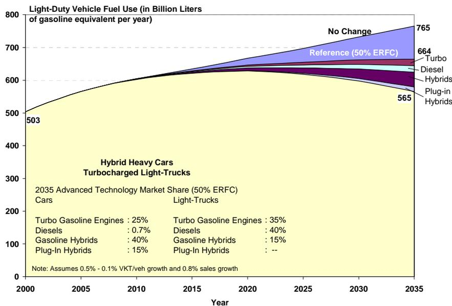
**Figure 62** LDV fleet fuel use under the combined *Hybrid Strong Scenario* in cars and the *Turbocharged Light-Trucks Scenario* in light trucks
