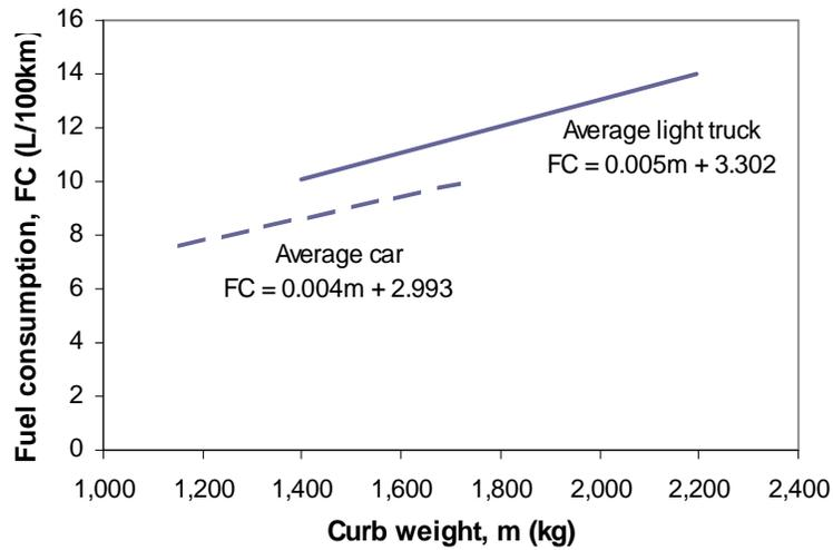
**Figure 13** Simulation results: curb weight-fuel consumption relationship for today’s vehicles
