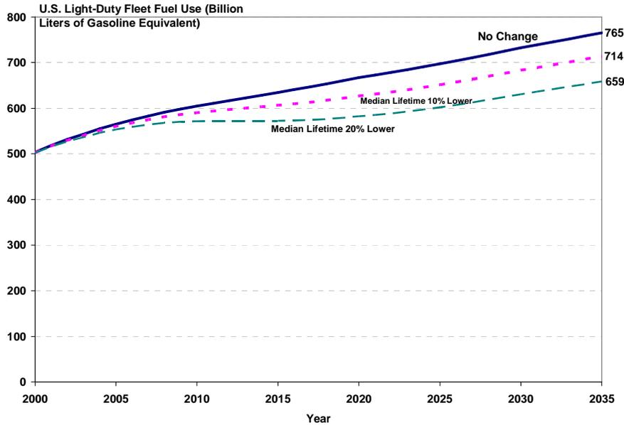
**Figure 34** Effect of reducing vehicle lifetime on fleet fuel use
