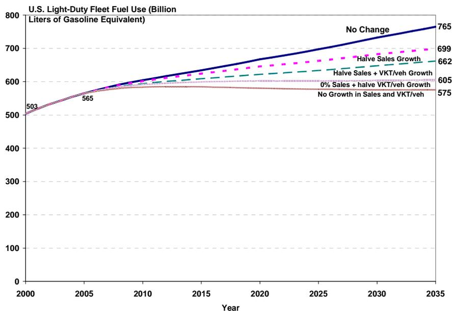
**Figure 33** Light-duty vehicle fleet fuel use projections for different sales and VKT/vehicle growth rates (2000–2035)
