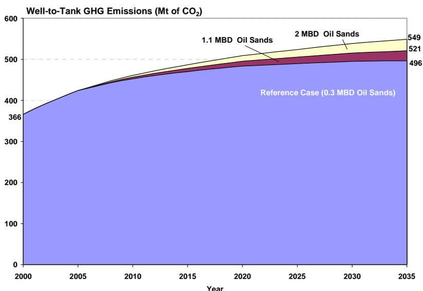
**Figure 45** Impact of increasing oil sands on well-to-tank GHG emissions
