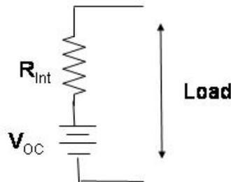
Figure 64: Battery equivalent circuit
