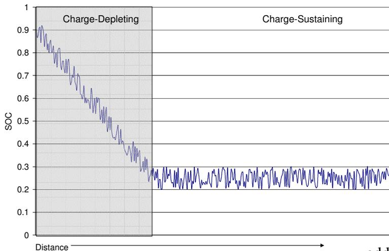
**Figure 7: Illustration of a typical Plug-In Hybrid duty cycle**
