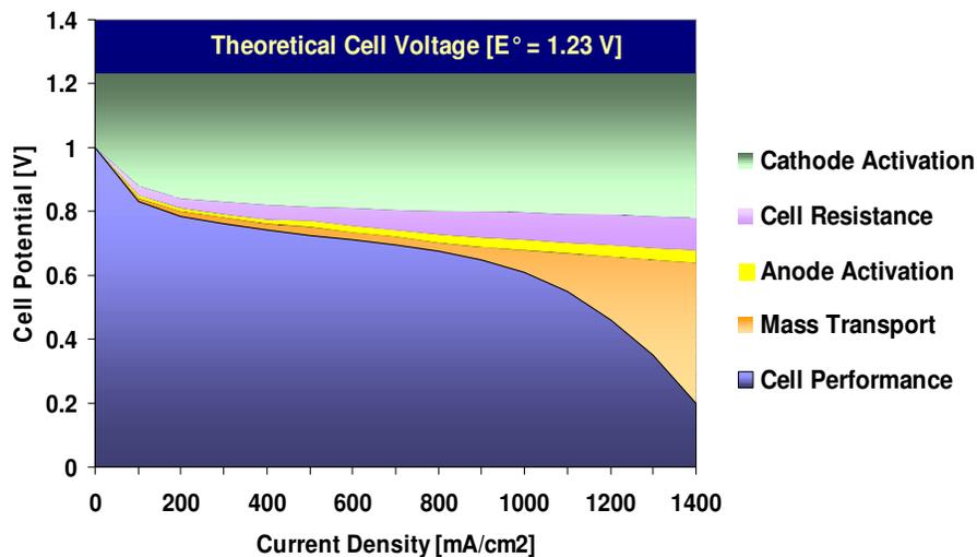
Figure 43: Illustration of fuel-cell stack losses [Frost 2006]
