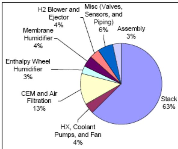
**Figure 51: Breakdown of balance-of-plant costs. Source: Carlson 2005**
