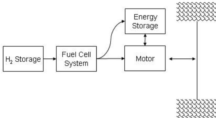
**Figure 41: A series-hybrid fuel-cell vehicle architecture. Arrows show possible power flows: The fuel-cell converts hydrogen to electricity, which is used to either deliver traction power to the motor or to charge the battery; a portion of the vehicle's kinetic energy may be recovered through regenerative braking.**
