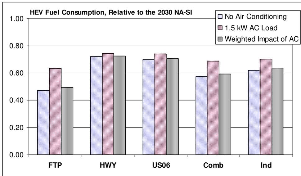
**Figure 20: Impact of air conditioning loads on hybrid vehicle fuel consumption**
