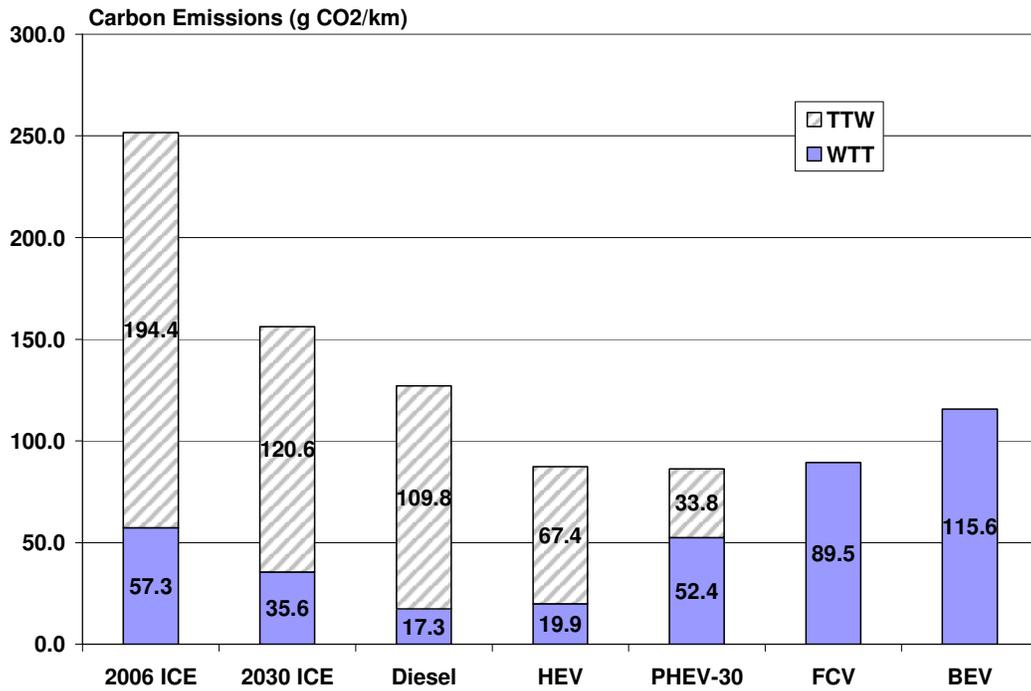
Figure 53: Well-to-wheel GHG emissions for different vehicle technologies.
