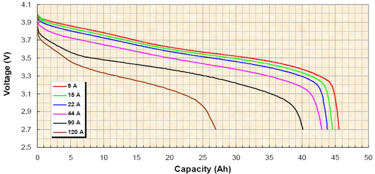
Figure 63: Saft VLE Discharge curve. Source: [Barsacq 2005]
