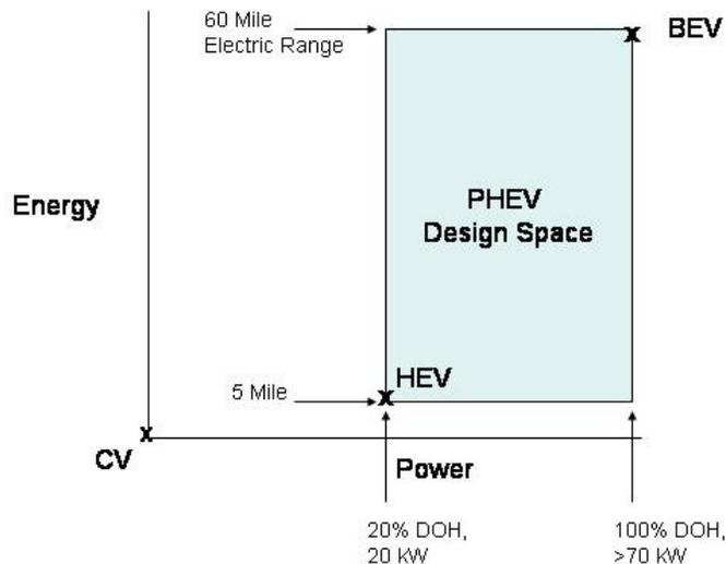
**Figure 24: Qualitative representation of the PHEV design space**
