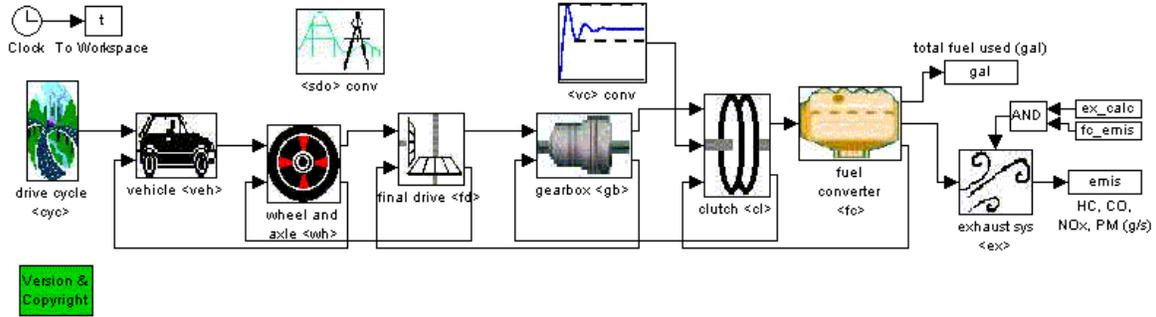
**Figure 5: ADVISOR Simulink block diagram.**
