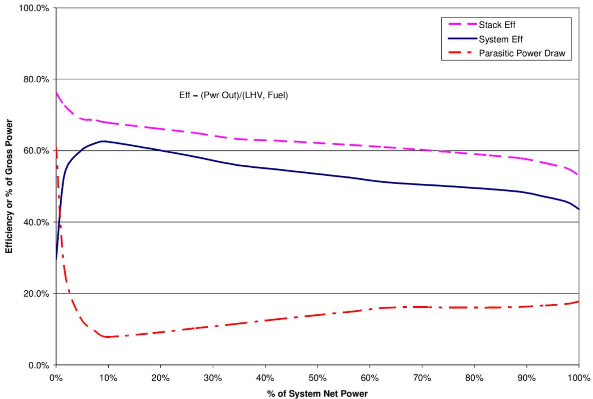
**Figure 47: Fuel-cell stack and system efficiency for the conservative case. Assumes the balance-of-plant does not include an expander module, and that the system rated power occurs at 0.60 V and 1500 mA/cm<sup>2</sup>.**
