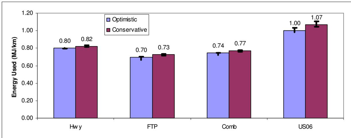
**Figure 52: Energy use for the fuel-cell vehicle for different drive cycles. The baseline vehicle uses a 40% hybridization ratio; the error bar shows the sensitivity to hybridization. The high-end energy use represents 25% hybridization ratio; low-end is 60% hybridization ratio.**
