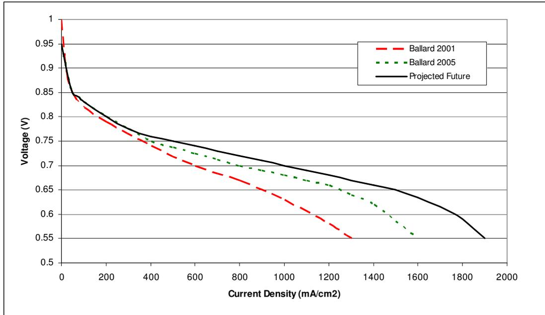
**Figure 44: Evolution of fuel-cell polarization curves. Historical data from [Guzy 2006].**
