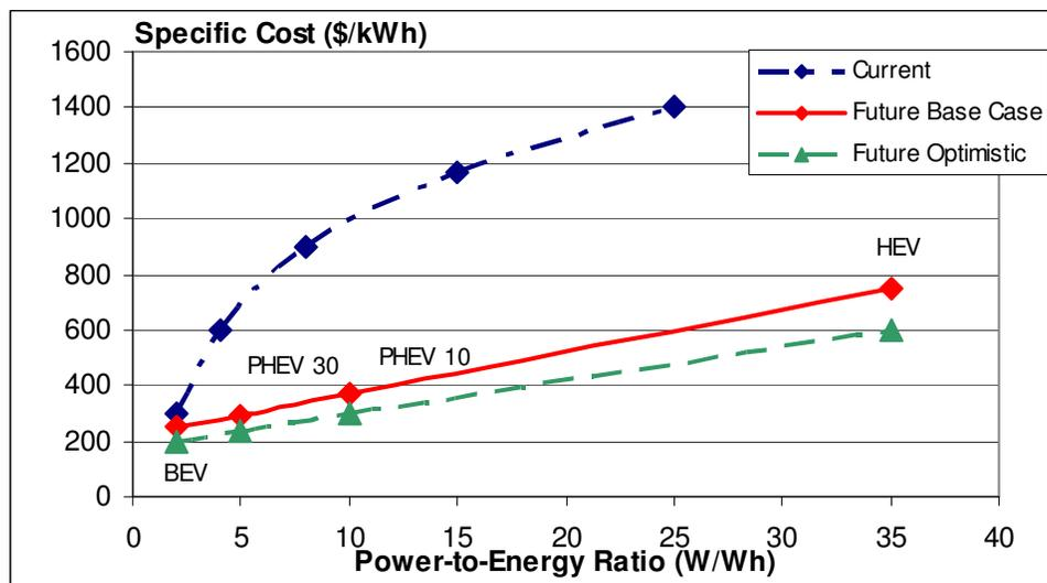
Figure 15: Current and future battery cost as a function of battery rate capability. Current data is based on a review of industry data and private correspondence [Miller 2007, Anderman 2000, Anderman 2005].
