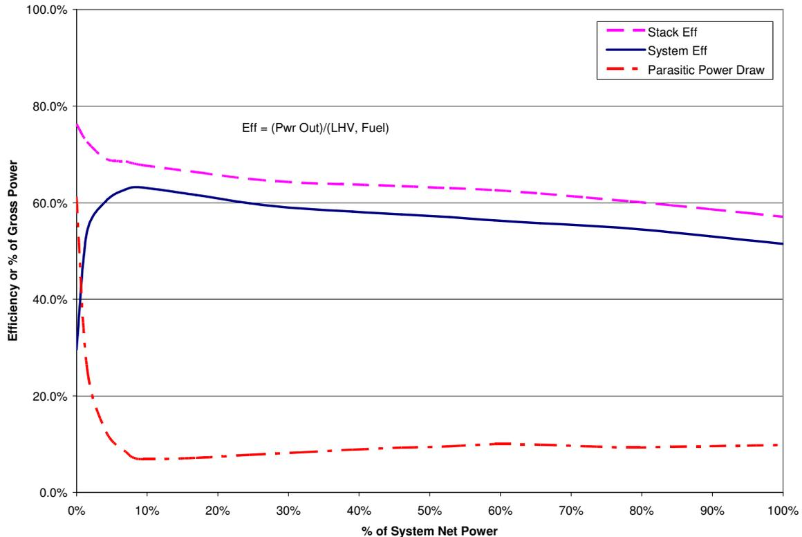
**Figure 46: Fuel-cell stack and system efficiency for the baseline case. Assumes the balance-of-plant includes an integrated compressor-expander module, and that the system rated power occurs at 0.65 V and 1500 mA/cm<sup>2</sup>.**
