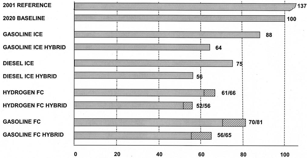
Figure 4: Relative life-cycle consumption of energy for vehicle technology combinations. Total energy (LHV) from all sources consumed during vehicle lifetime shown as percentage of baseline vehicle energy consumption. Total energy includes vehicle operation and production of both vehicle and fuel.
