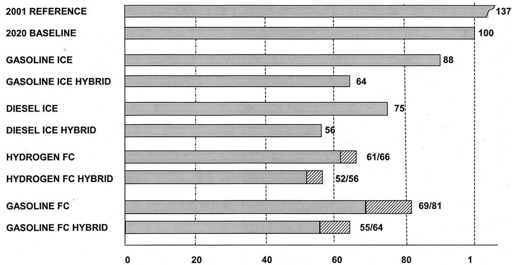
Figure 5: Relative emissions of life-cycle greenhouse gases for vehicle technology combinations. Total mass of carbon equivalent emitted during vehicle lifetime shown as percentage of baseline vehicle GHG emissions. Greenhouse gases include only CO<sub>2</sub> and CH<sub>4</sub> (assumed equivalent to 21 CO<sub>2</sub>). Emissions include vehicle operation and production of both vehicle and fuel.
