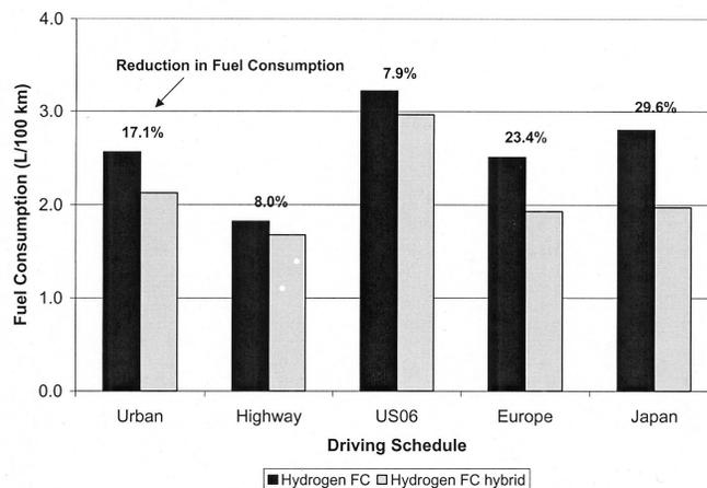
Figure 3 shows the results for the advanced fuel cell and fuel cell hybrid vehicles. The trends are similar, but the percentage hybrid fuel consumption benefits are significantly lower. Since the fuel cell is relatively more efficient at lighter loads, whereas the ICE exhibits the reverse trend, this part of the hybrid benefit (shifting the “engine” to higher loads) is much reduced.
