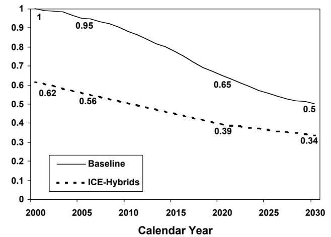
Figure 6: Relative Improvement in fuel consumption (vertical axis) relative to the 2000 new car average fuel consumption.
