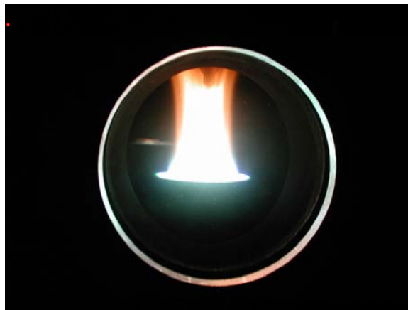
Figure 10: A sooting flame (right) generated in the Howard laboratory at MIT to study soot formation in flames. The yellow tinge denotes radiation and the presence of carbon particles.
