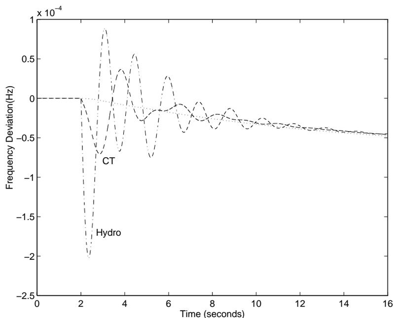
Figure 13: Hydro Gate Opening Time Constant Increased
