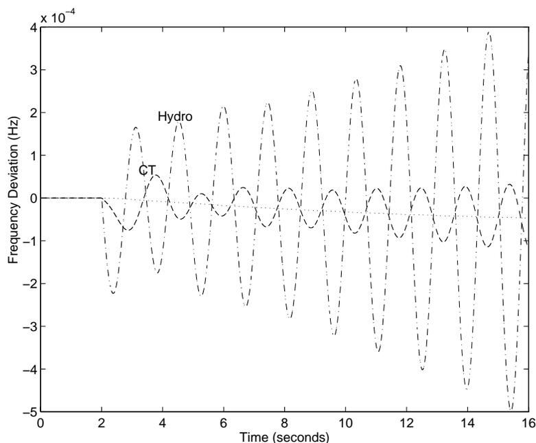
Figure 12: Frequency Deviation with Hydroelectric and Combustion Turbines
