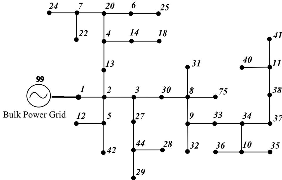
Figure E.2: 37 Bus Radial Distribution Test System
