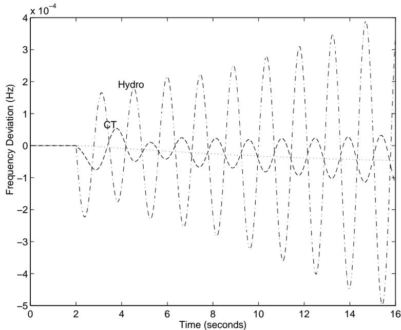
Figure B.10: Frequency Deviation from Equilibrium for Hydroelectric and Combustion Turbines substation.<sup>2</sup>
