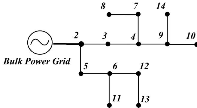
Figure E.1: 14 Bus Radial Distribution Test System
