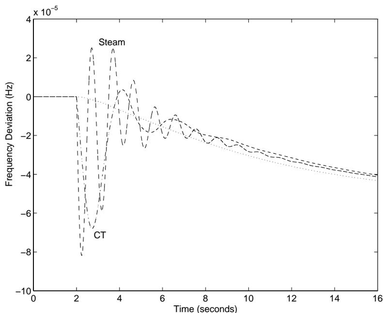
Figure 10: Base Case—Frequency Deviation After Load Deviation Turbine
