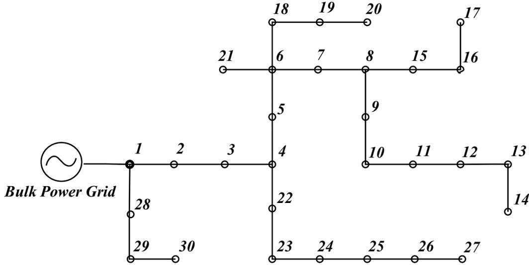
Figure B.6: 30 Bus Radial Distribution Test System
