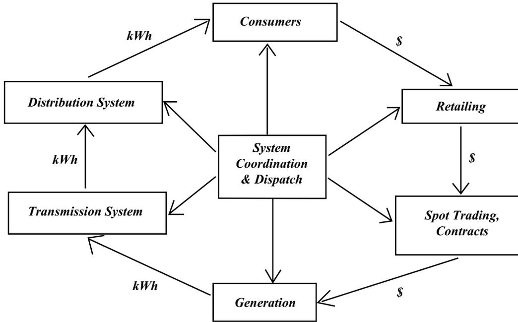
Figure C.3: Functional Blocks of the Electric Power Industry
