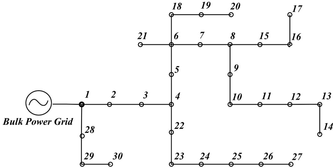
Figure 9: 30 Bus Radial Distribution Test System
