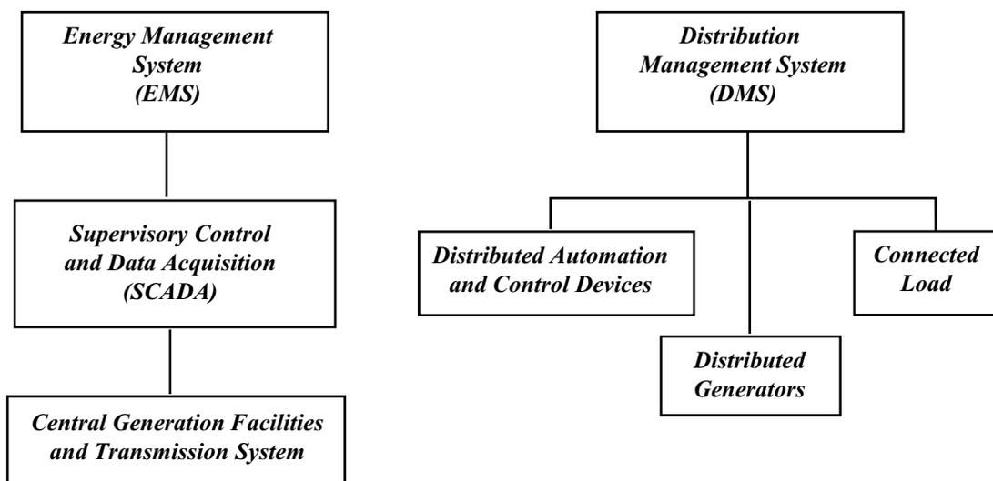
Figure A.3: Projected Structure for Combined Energy and Distribution Management Systems
