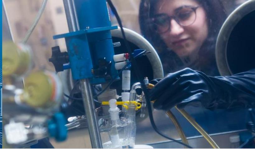
Graduate student Aliza Khurram prepares for experiments by pumping carbon dioxide through an electrochemical cell consisting of lithium and carbon electrodes plus a specially designed electrolyte. *Photo: Stuart Darsch*
