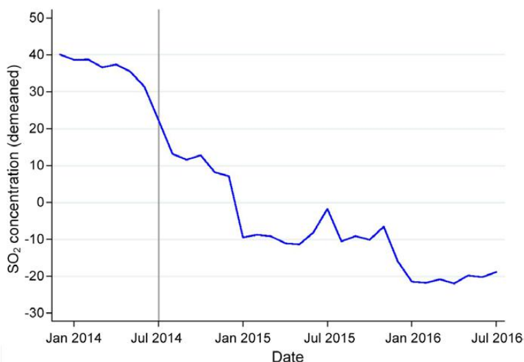
Adjusted SO 2 concentrations reported by a sampling of Chinese power plants This figure shows the monthly average of SO 2 concentrations measured by continuous emissions monitoring systems (CEMS) on the exhaust stacks of 256 power plants and reported by firms. To account for the different emissions levels across plants, the long-term average for each plant is normalized to zero. This curve shows emissions above or below that level on average for all plants. The figure shows a clear decline in emissions leading up to the July 2014 compliance deadline as well as following it.
