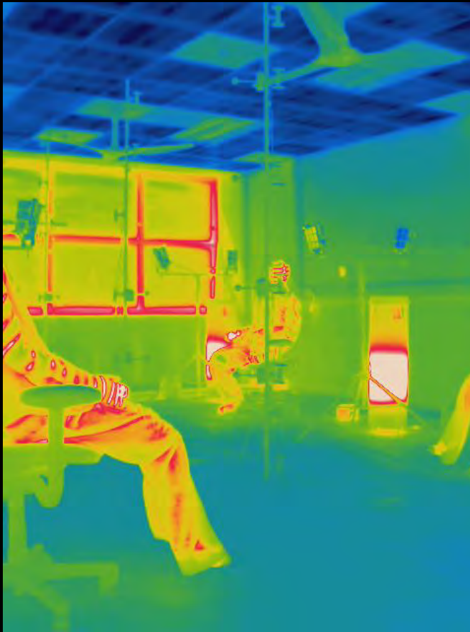
RADIANT COOLING (CEILING) OPERATIVE TEMP = 26° C
