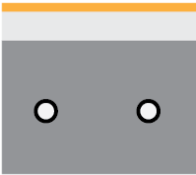
Thermally Activated Building System (TABS)
