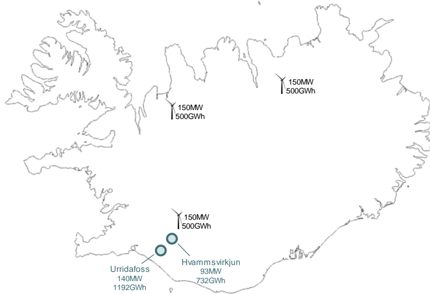
Figure 31: Generation investments in hydro and wind technologies in year 2030
