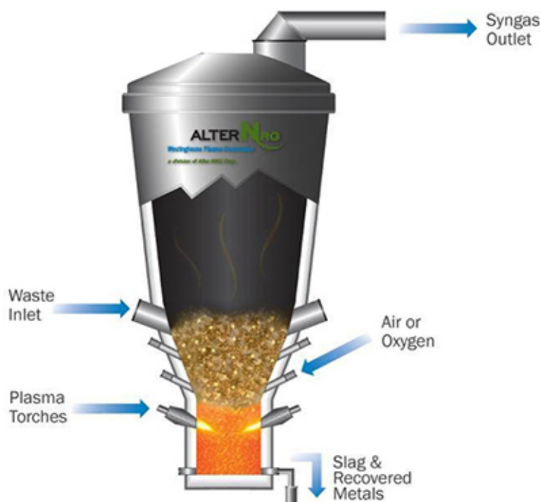
Figure 5.3 | AlterNRG (Westinghouse) plasma gasification technology [46].
