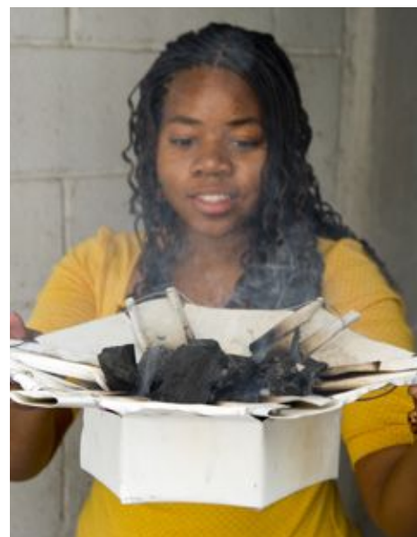
Julie Paul '10, a student in “D-Lab: Energy,” shows off her team’s prototype of a “stove-within-a-stove,” an insert fabricated of aluminum sheeting to enable residents of rural Nicaragua to substitute cleaner-burning charcoal for wood as a cooking fuel.
