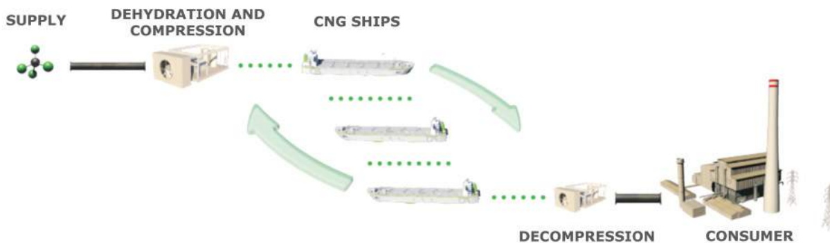
Figure 22 – Overview of a Compressed Natural Gas Delivery System
