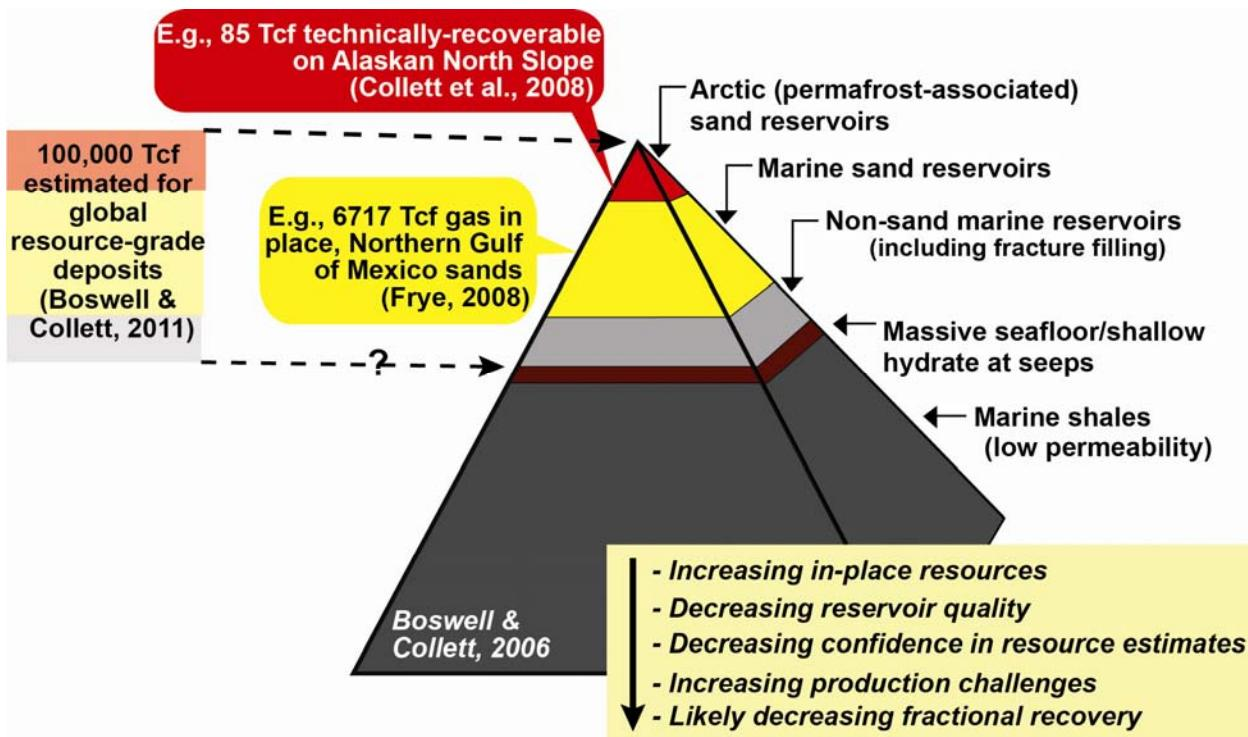
Figure 3. The hydrate resource pyramid modified from Boswell and Collett (2006).
