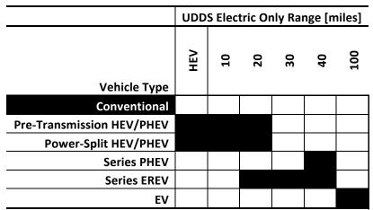
Table 1 – The vehicle design matrix: Filled cells mark vehicles under consideration.
