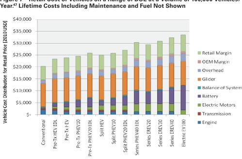
Figure 7 – Retail Cost of Vehicles on a Range of DOE at a Volume of 100,000 Vehicles/ Year.47 Lifetime Costs Including Maintenance and Fuel Not Shown
