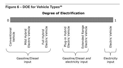
The most significant difference between these vehicles is in the drive train, comprising the set of components that produces vehicle propulsion. In a traditional ICE vehicle, the engine is the sole source of propulsion. Adding an electric motor to the drive train enables the use of electricity for propulsion, thereby creating three classes of vehicles: HEVs, PHEVs, and BEVs. In this paper, the term "EV" refers to PHEVs and BEVs.
