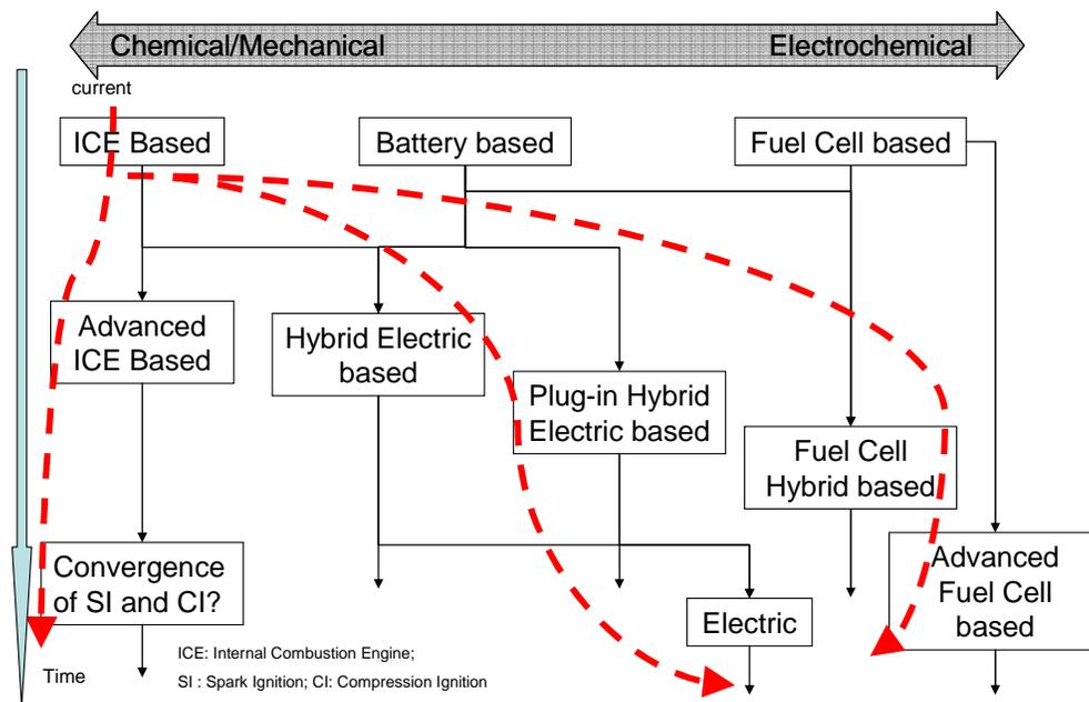
**Figure 8** Possible propulsion system pathways
